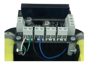
Take the wires from the motors and connect them to the terminal blocks on the motor driver board in the following configuration:
