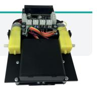
Attach the red and black wires into the terminal on the Motor Driver Board labelled 'POWER'. Put the black wire in the left hand side of the terminal labelled 'BLACK' and the red wire in the right hand side of the terminal labelled 'RED'. Finally slide the wheels onto the motors and get coding!
